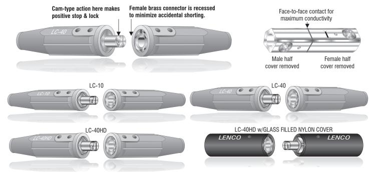
The glass filled nylon covers are designed for extreme heat and impact resistance applications.
