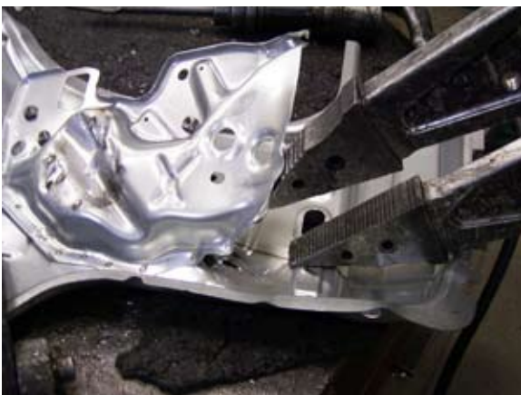
Spot-weld integrity testing is completed by ripping the seams apart with a LUKAS LSI combi tool or LUKAS spreader. The spot weld rip-pattern provides feedback on the optimal settings for the weld robots.
