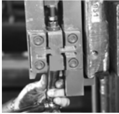
Figure 4-29. Loosen and Remove Bottom Hex Nut
