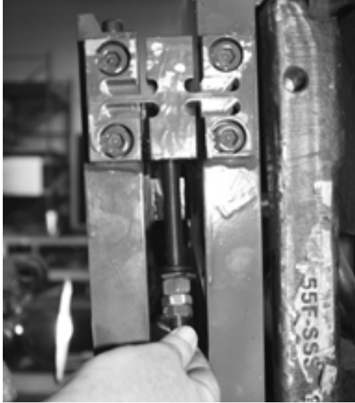
Figure 4-34. Installing Flexure into Scale
