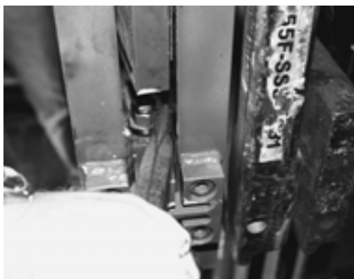
Figure 4-38. Centering the Load Cell Using a Chisel
