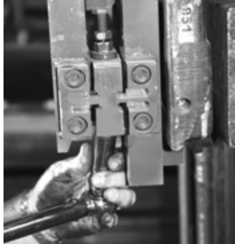
Figure 4-39. Tightening the Lower Hex Nut
