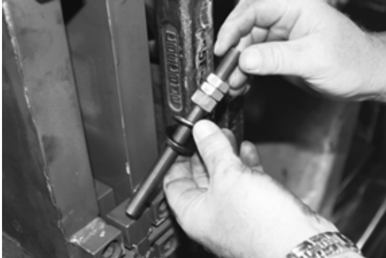
Figure 4-36. Install Spherical Washer Set
