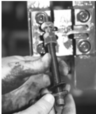
Figure 4-30. Remove Flexure Rod with Nuts and Washers
