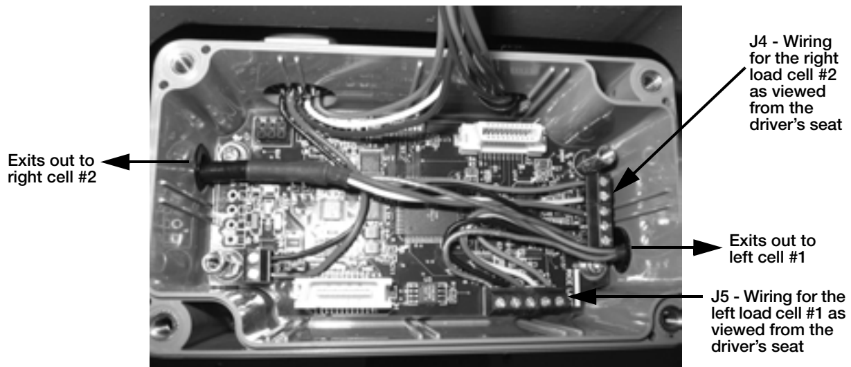
Figure 4-17. Bottom Board Wiring
