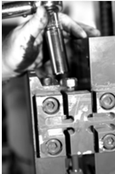
Figure 4-28. Removal of Hex Nut
