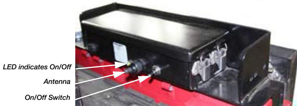
Figure 2-20. Wireless Battery Option
