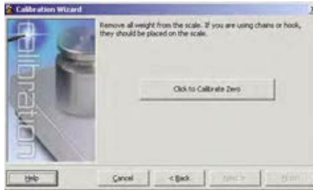
Figure 5-10. iRev 4 Zero Calibration Display
