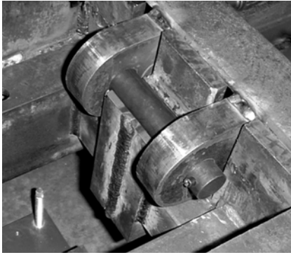
Figure 2-3. Pin and Receptacle Interface
