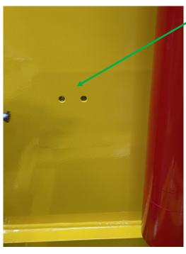
Hinge block fixing holes in clamping frame
