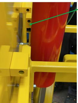
Using an assistant offer-up main frame of guard to hinge blocks
