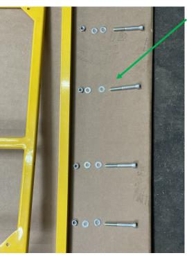
Actuating arm fixings M8 x 70mm socket caps, nuts and washers
