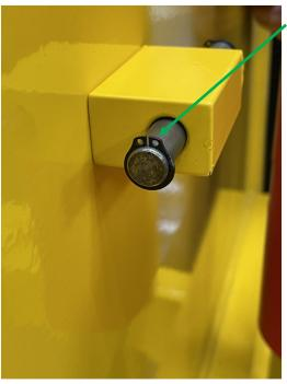
Remove circlips and hinge pins
