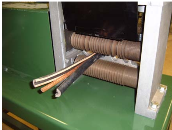
Figure 4-5 Cable wire finish cut.
