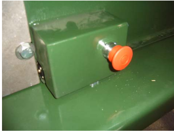
Figure 4-3, Emergency Switch (Red) and Contact Switch
