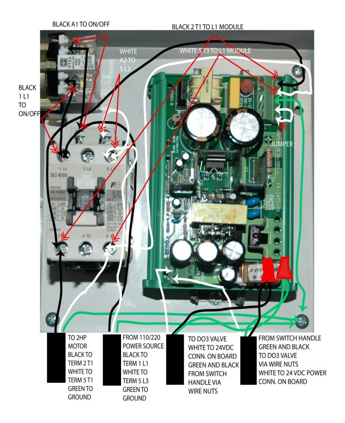
110 WIRE DIAGRAM W/ POWER SUPPLY MODULE
