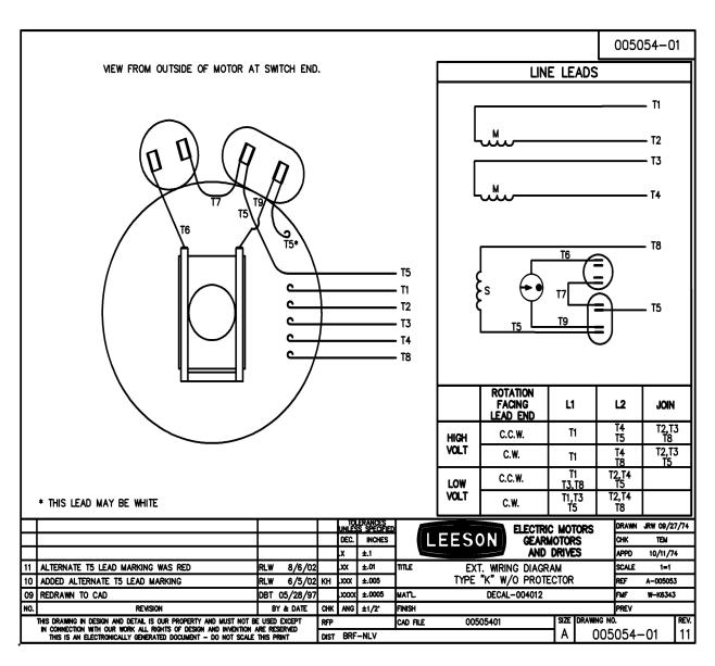
LEESON 2HP INTERNAL WIRING LOW VOLTAGE FOR 110 MODEL HIGH VOLTAGE FOR 220 MODELS
