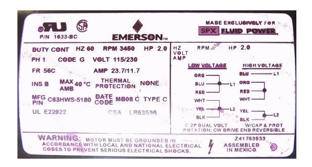
WIRING DIAGRAM FOR THE EMERSON 110/220 MOTOR, FOR 110:
