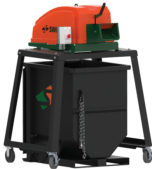
The Model 450 DDX is shown sitting on and over an optional basic stand and 1/2 yard self-dumping hopper.
