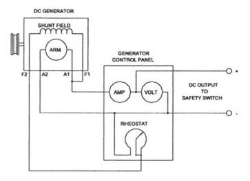
Connections on generator shown for C.C.W. rotation facing commutator end. Interchange field connections for clockwise rotation.
