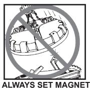
**DOWN EASY** Ease your magnet down onto the material. Repairs are costly and lost
