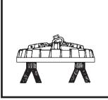
**KEEP MAGNET DRY** Always store magnet off of the ground. Never cool the magnet with water. Store in dry area - moisture can cause short circuits thereby crippling lifting capacity.
