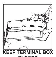
**CLOSED** This keeps moisture away from the terminals and out of the magnet coil..
