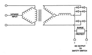
Rectifier must be rated for magnet service and be equipped with surge protection.
