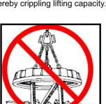
KEEP POWER OFF UNTIL MAGNET SETTLES ON LOAD
