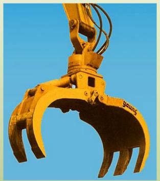
An all purpose tool for handling loose scrap metal, car bodies, demolition debris and more. Features two opposing tines with multiple tips allowing the tines to bypass resulting in a tight squeeze on bulky materials and long objects.
